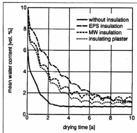
used. While the polystyrene has the highest U-value this wall also takes the longest to dry-out (10 years). The plaster takes 6 years and the mineral wool seven. The slower times relate directly to the varying abilities of the insulants to allow vapour move through them into the room. The polystyrene used was 23-times more resistant to vapour diffusion than the mineral wool.
