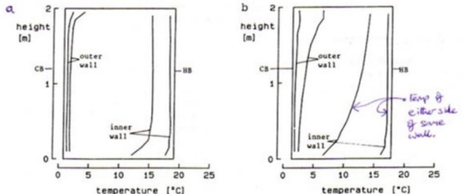
Heat Loss method in TGD L gives an air cavities a Resistance value of 0.180m2K/W regardless of its width (or any gaps) an enthusiastic estimator might count *both* voids and expect an even better U-value than 0.34W/m2K!
